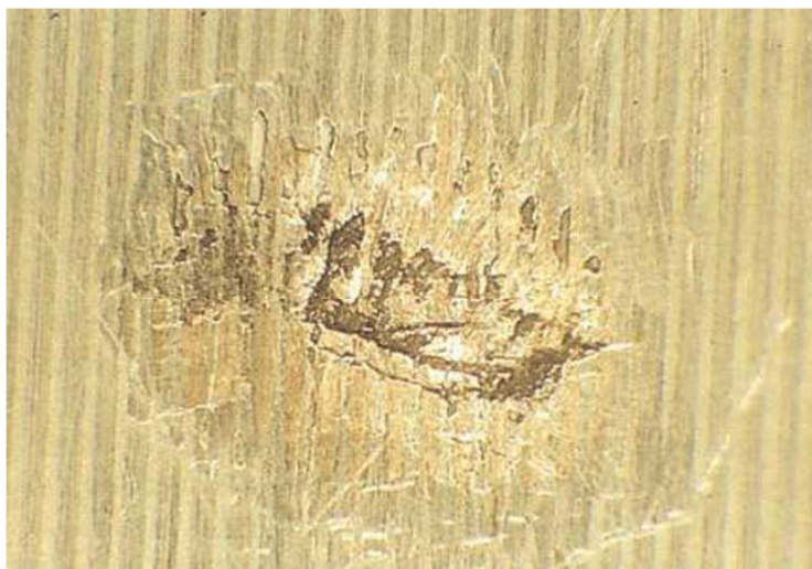
Fig. 9 Chip Embedded in the Surface of a Friction Bearing
