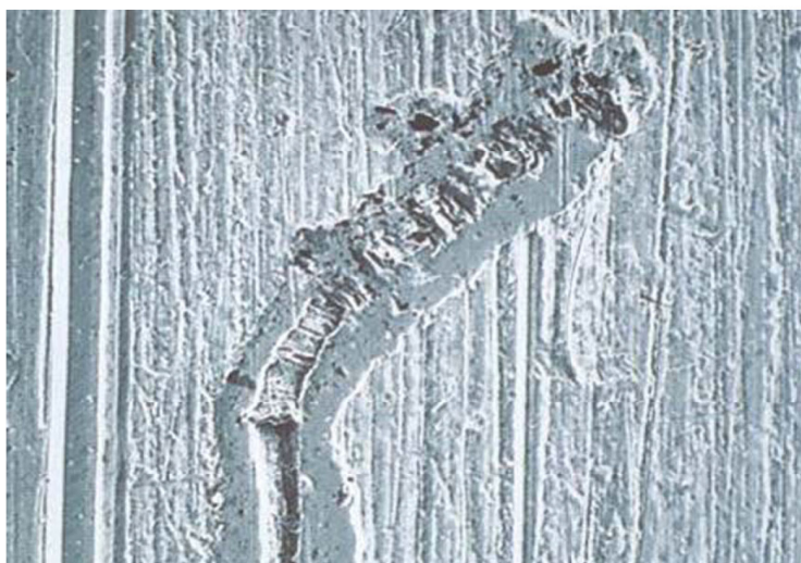
Fig. 9 Chip Embedded in the Surface of a Friction Bearing
