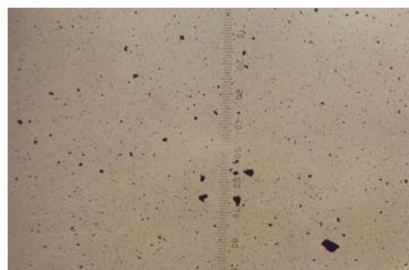
Fig. 12 Microscopic Examination of an Oil Sample (100 ml) Magnification 100x (NAS 10)
